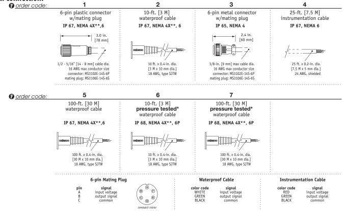
\*-Test pressure: 100 feet [30 meters] H<sub>2</sub>O (40 PSID); Test Medium: Air; Duration: 2 hours. \*\*-Applies to stainless steel enclosure only.
