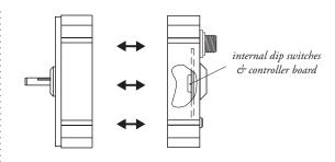
To gain access to the signal board, remove four Allen-Head Screws and seperate the two case halves.
