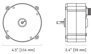
The RT9510 is an incredibly simple device which provides a regulated 0...10 VDC rotational-position feedback signal with a 14.5...40 VDC unregulated input voltage.
